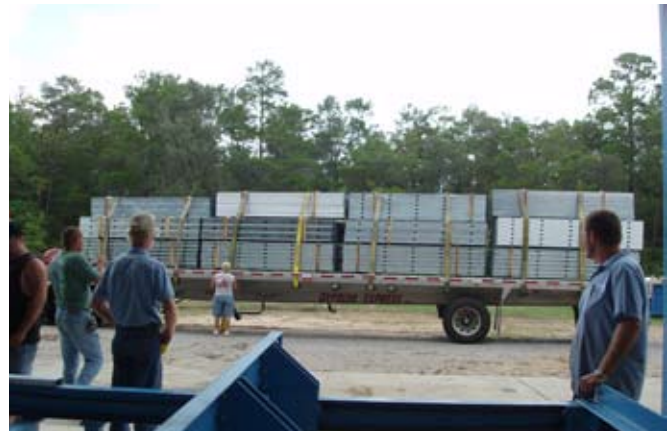
Finished steel framing products are stacked into bunks and loaded onto trucks.
