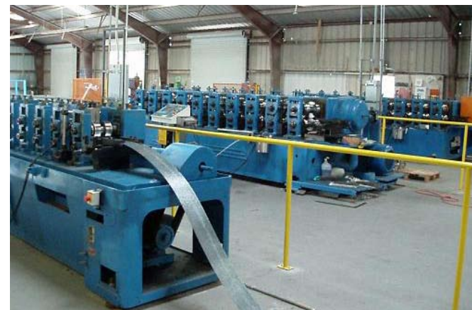
Roll-forming operations produce steel framing products. Southline Steel operates 8 roll-form lines in Alabama and Florida.
