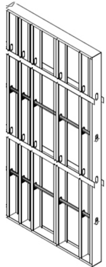
Load Bearing Wall braced with CRC and flat strap.
