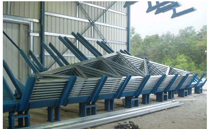
Floor and roof trusses are designed in Freeport, FL. Trusses are assembled at plant locations in Alabama and Florida. Shown is roof truss assembly table in Freeport, FL.
