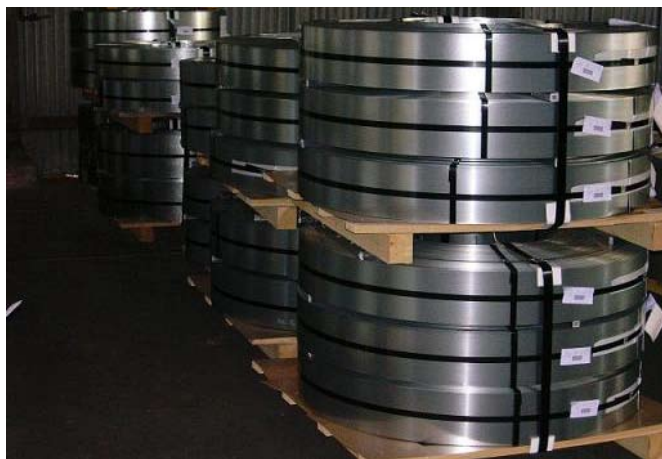
Slitting operations in Bessemer cut primary coil into multiple coils for roll-forming.
