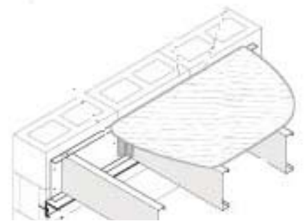
Structural Stud used as Floor Joist Application - 2.
