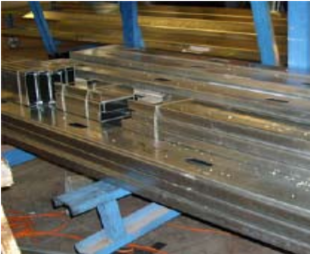
Step 1. Truss material comes off the assembly line cut to length and machine-labeled. The material for each truss is stacked and staged on movable carts and staged for assembly.
