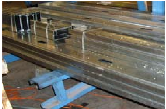
Step 1. Truss material comes off the assembly line cut to length and machine-labeled. The material for each truss is stacked and staged on movable carts and staged for assembly.
